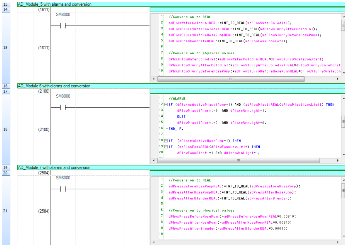
Figure 20, GX Works 3, handling of AD-values.
