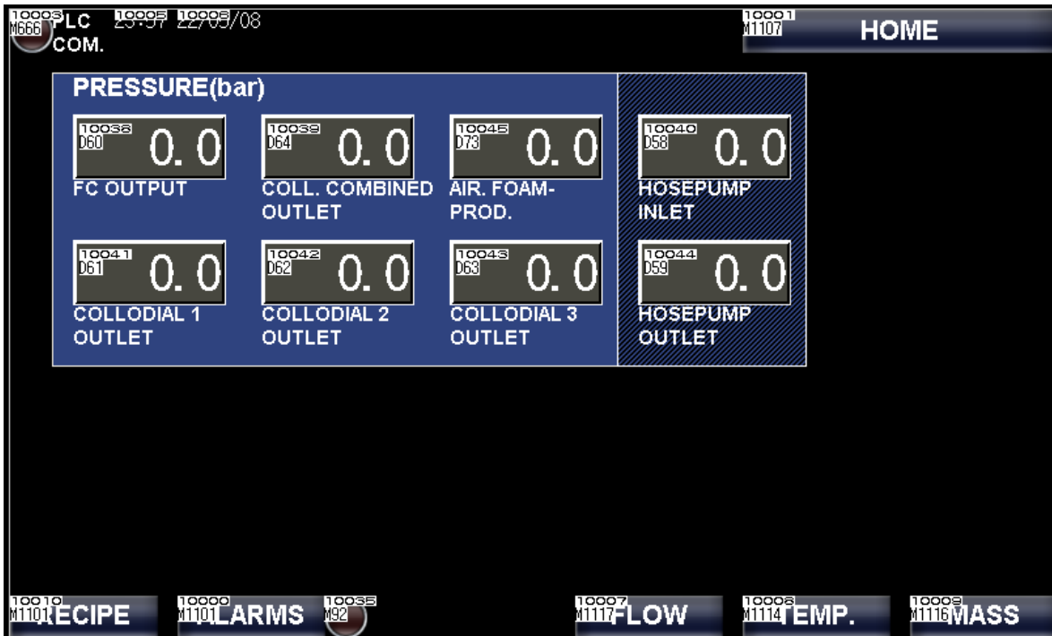
Figure 16, Screen, GT Designer 3, displaying data, pressure screen.
