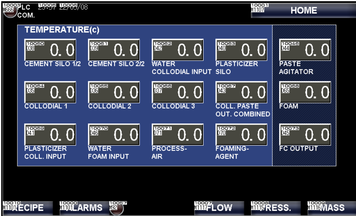
Figure 15, Screen, GT Designer 3, displaying data, temperature screen.
