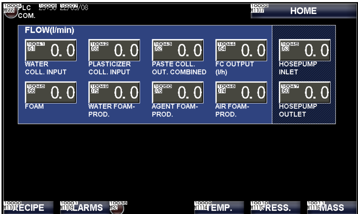
Figure 14, Screen, GT Designer 3, displaying data, flow screen.
